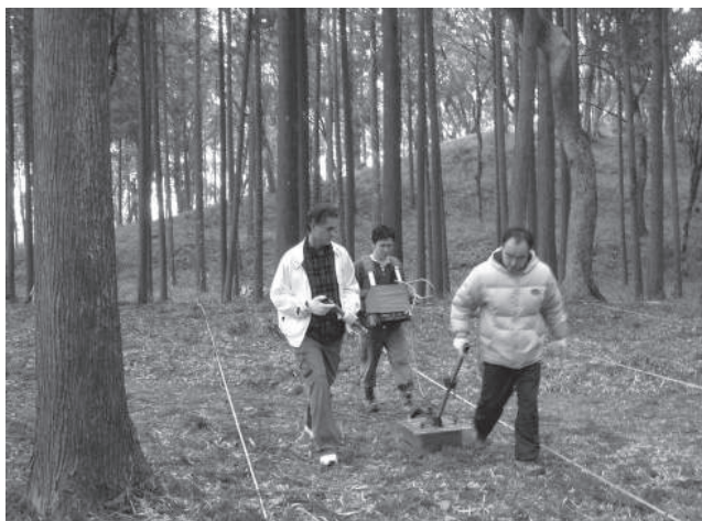
Figure 2: GPR surveying with a 500 MHz antenna at the Osaho-Mesaho Kofun mounds.
