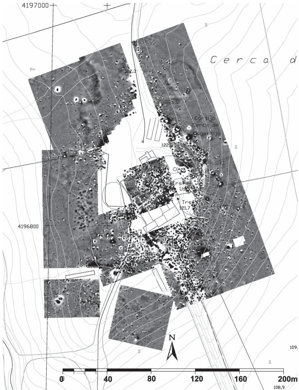
Figure 3: Roman settlement and illegal waste dump. Geomagnetic map of the Cortijo de Lagartijo area (PP-LE1). Dynamics: \pm 15 nT/m.
