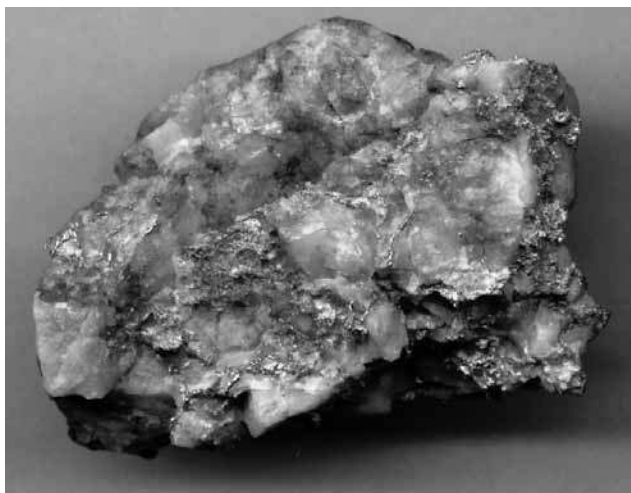
Figure 1: (See colour plate) Gold (fineness 885) in quartz vein. 81 mm. Bestube, Northern Kazakhstan. Collection and photography – E.S. Perhaps this deposit was one of the gold sources for the well known ancient Scythian jewellery.
