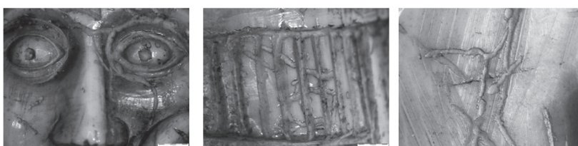
Figure 7: (a) post polishing damage channel on the cheek and (b) carved hair. The channels cross rather than branch (c).
