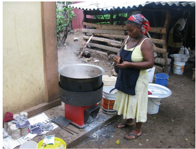
Figure 3. Fuel-efficient institutional stove using locally made biomass briquettes in Haiti Credit Prakti
