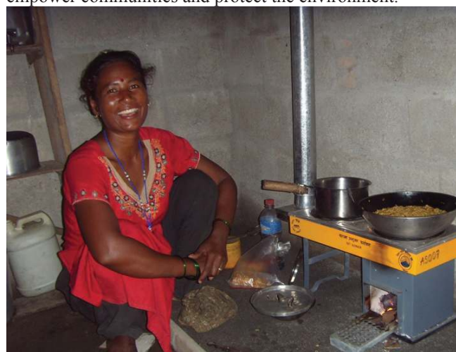
Figure 2. Improved double pot stove in Nepal with 50% fuel consumption and no harmful emissions
