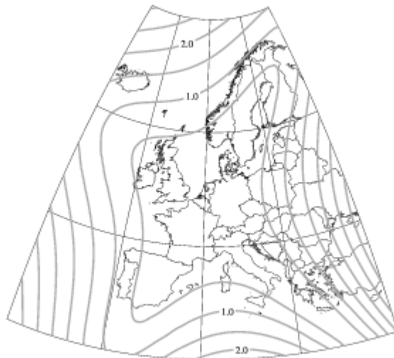
Figure 3. Fifth-order low-error transformation of the oblique azimuthal equal-area projection for the European Union, with lines of constant maximum scale error (%).
