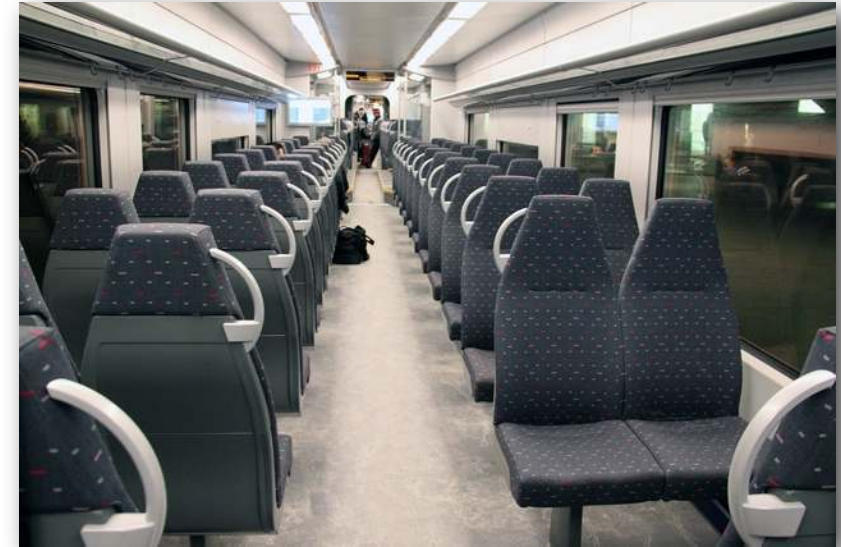
Figure 2. Interior (second class) of a SNCB Siemens Desiro ML train already in service. Note the density of the layout and the lack of tables. Source: photo Maurits90 via Wikimedia, Creative Commons - certain rights reserved.
