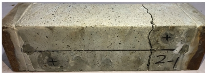
(a) RSCC-0 specimen with no rubber particle content
