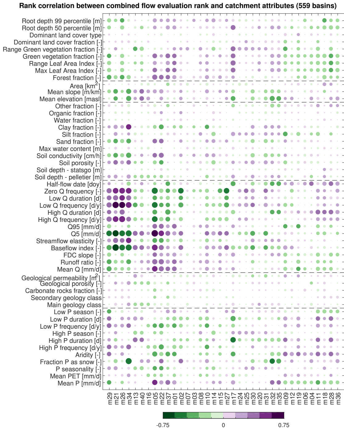
Figure C.13: Spearman rank correlation between model ranks (obtained during combined flow ( \frac{1}{2}[KGE(Q) + KGE(1/Q)] ) objective function evaluation) and CAMELS catchment attributes. Models are ranked from best to worst, with rank 1 indicating the best model. Only correlations with p-value < 0.05 are shown. Marker size corresponds to the strength of the correlation, as does the intensity of the colours. Models are sorted manually in an attempt to place models with similar correlation patterns close together. The sorting order is the same as used in Figure C.14.
