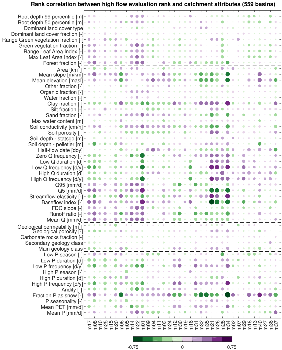
Figure C.10: Spearman rank correlation between model ranks (obtained during high flow (KGE(Q)) objective function evaluation) and CAMELS catchment attributes. Models are ranked from best to worst, with rank 1 indicating the best model. Only correlations with p-value < 0.05 are shown. Marker size corresponds to the strength of the correlation, as does the intensity of the colours. Models are sorted manually in an attempt to place models with similar correlation patterns close together. The sorting order is the same as used in Figure 9. This makes the models with snow components stand out slightly. See m06, m12, m30 and m37 which would here be better placed near models m31, m32, m35, m21 and m26.
