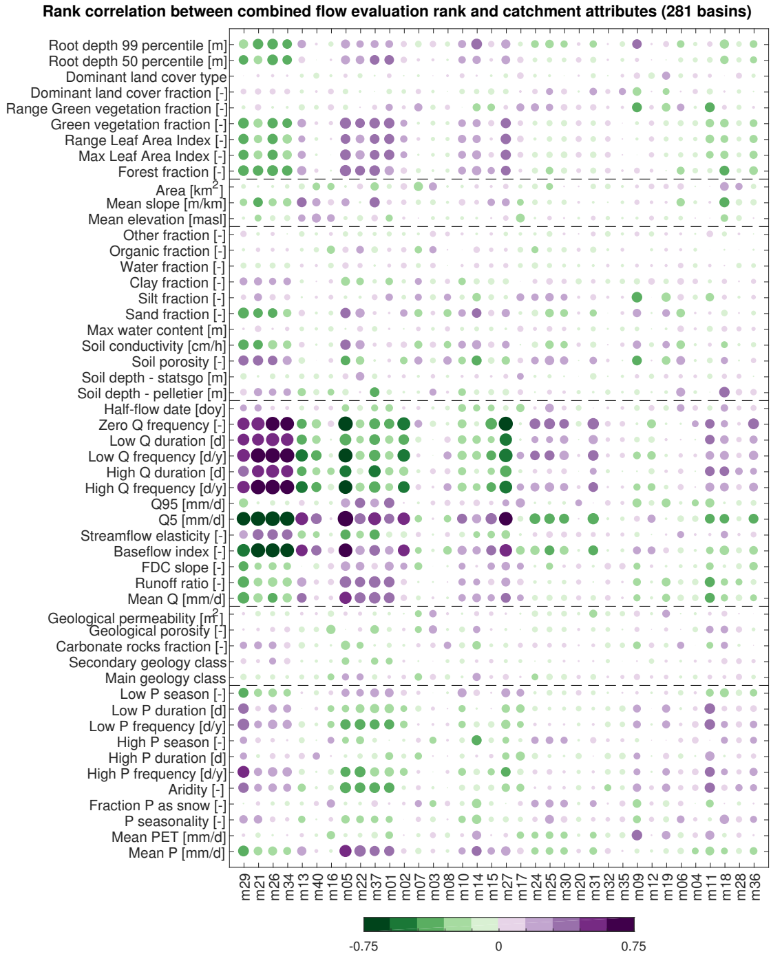
Figure C.14: Spearman rank correlation between model ranks (obtained during combined flow ( \frac{1}{2}[KGE(Q) + KGE(1/Q)] ) objective function evaluation) and CAMELS catchment attributes. Only catchments where less than 10% of annual precipitation occurs as snowfall are included in this figure. Models are ranked from best to worst, with rank 1 indicating the best model. Only correlations with p-value < 0.05 are shown. Marker size corresponds to the strength of the correlation, as does the intensity of the colours. Models are sorted manually in an attempt to place models with similar correlation patterns close together. The sorting order is the same as used in Figure C.13.
