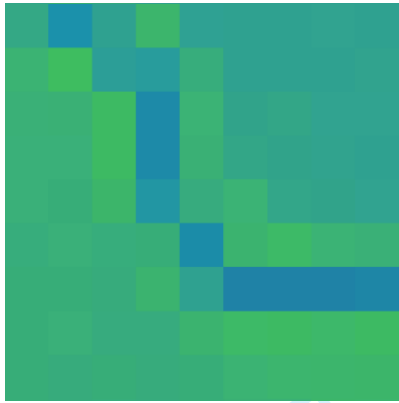
Figure 11. 25m resolution DEM. Dark blue - canal, light green – levee.
