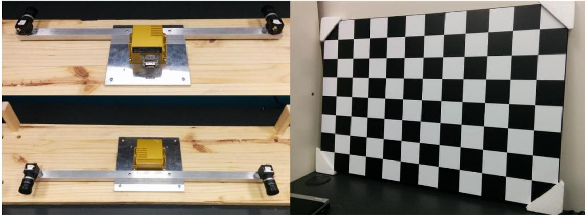
Figure 4.12 Stereo Camera System with IMU (Left). 90x60cm Checkerboard (right)
