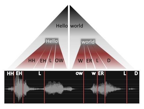
Figure 2.7: An illustration of the text to speech process. A text structure is converted into words. Each word into phonemes. And for these to an actual audio signal.
