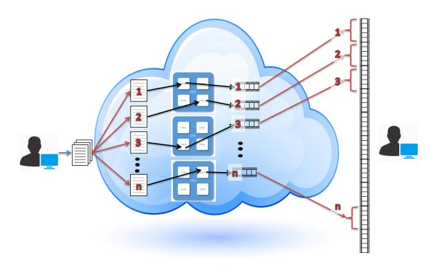
Figure 2.9: A illustration of cloud based rendering. A rendered sequence can be parallelized and then re-integrated into a coherent video sequence.
