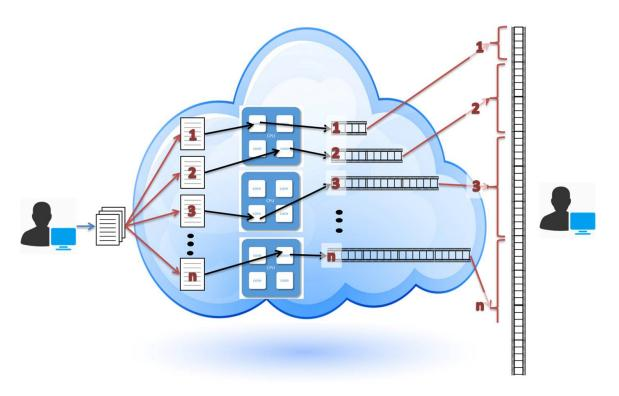
Figure 5.2: The multi-process rendering system. A clip to be rendered is split into non-uniform length pieces and distributed to the rendering farm. The rendered sections are pieced together in the correct display sequence.
