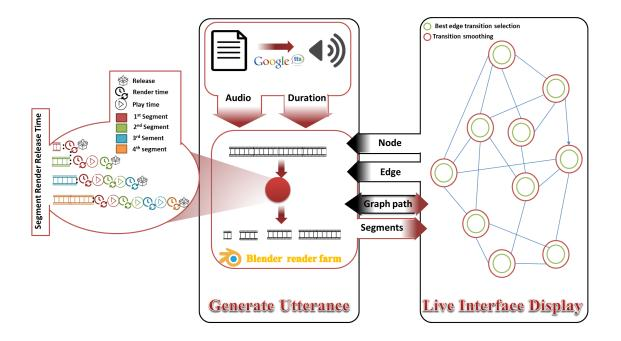
Figure 5.1: A parallel multiprocess generation of the utterance to reduce latency in display. under the assumption that  $T_p = kT_r$  then  $T_r^n = T + k \sum_i^{n-1} T_r^i$ .
