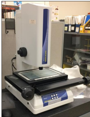
Figure 5: Mitutoyo Quick Scope Vision Measuring System
