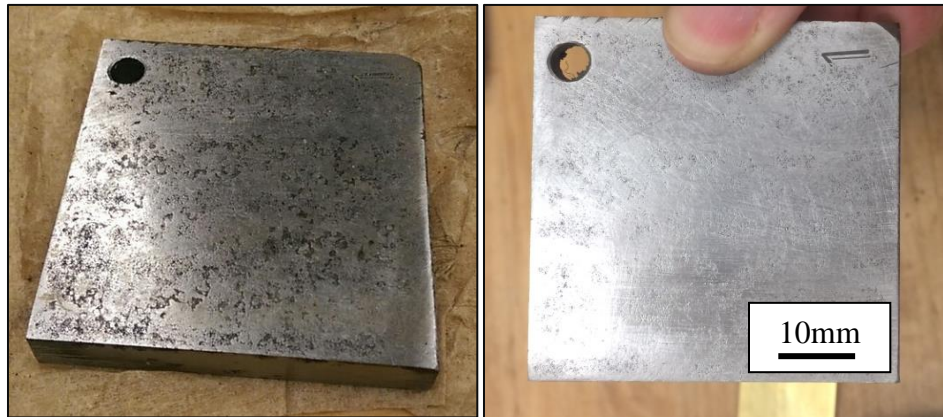
Figure 2: Steel sample before and after sanding.
