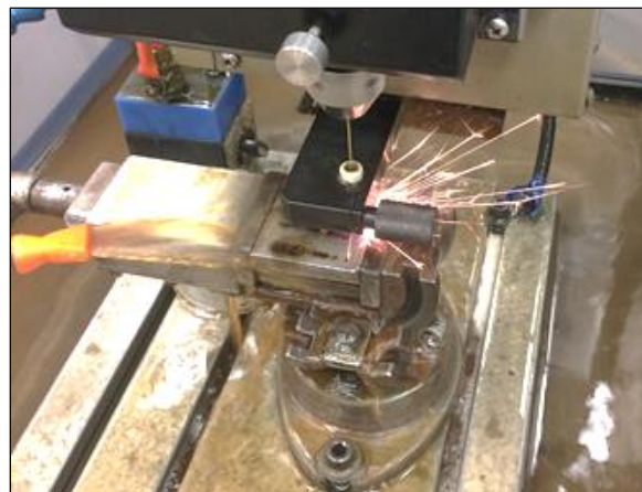
Figure 4: EDM'ing on a steel workpiece.
