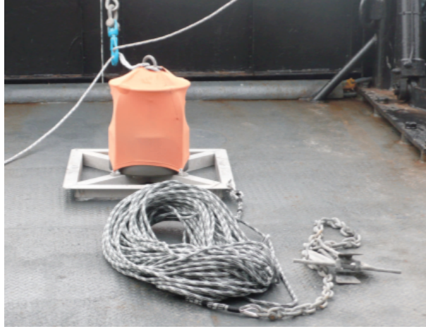
Figure 1.5: Example of one Directional Autonomous Seafloor Acoustic Recorder (DASAR).
