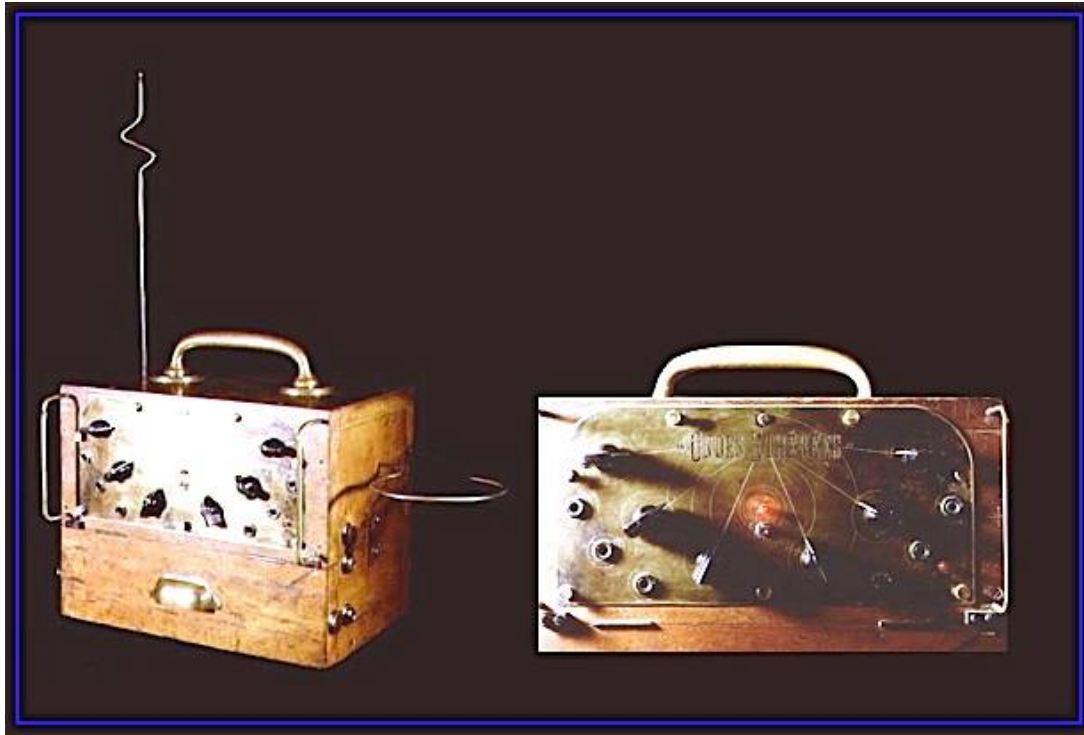
Fig. 2: A rare photo of an instrument that matches Loriod's description of one of the earliest Ondes Martenot models. The instrument has 'Ondes Éthériques' on the front
