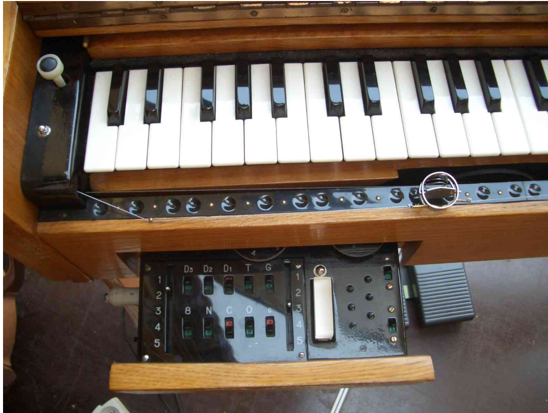
Fig. 7: The drawer, or tiroir, of a model 7 Ondes Martenot, with the ten switches for timbre and diffusers to the left of the volume button
