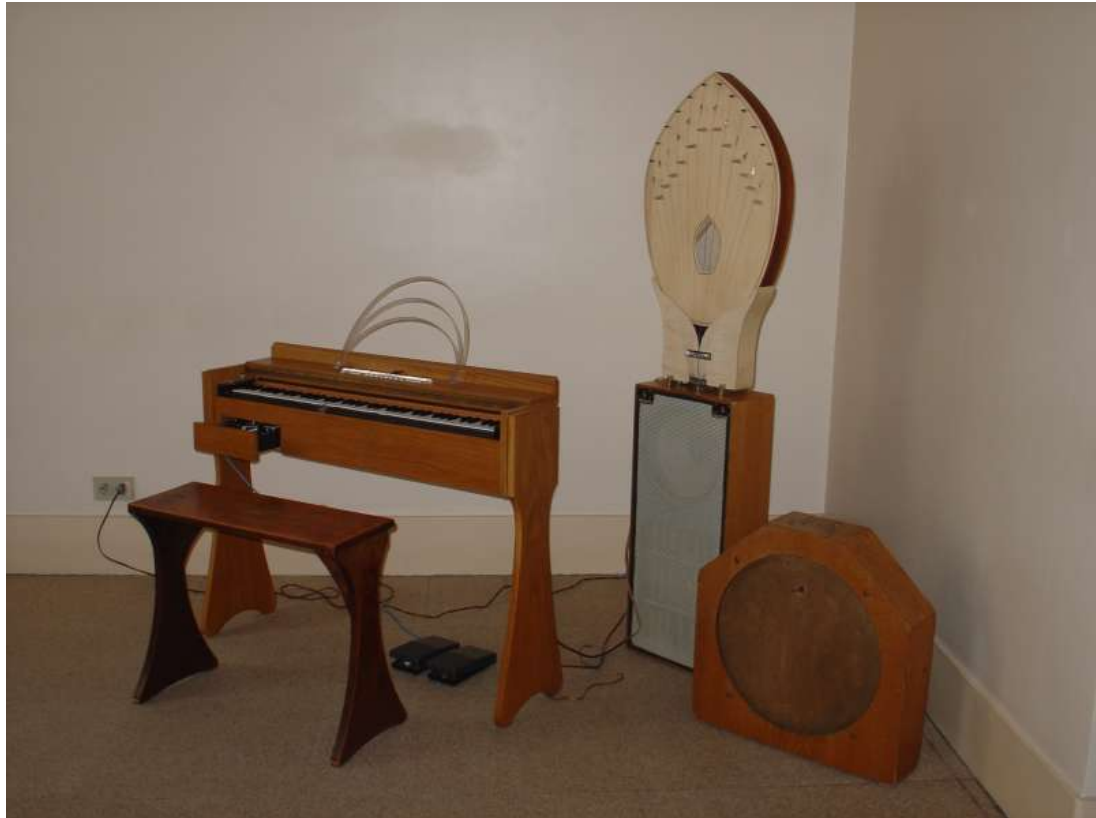
Fig. 8: The setup of the Ondes Martenot model 7: main instrument with 6-octave keyboard, résonance diffusor with palme diffusor on top, and the métallique to the right
