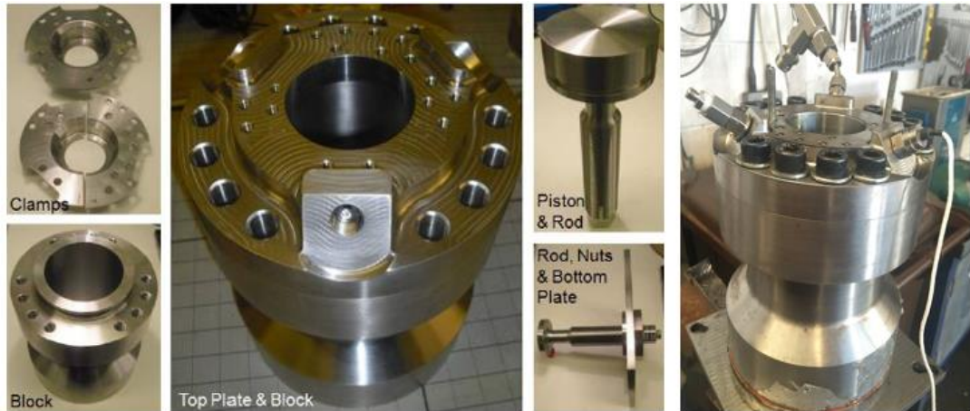
Figure 3.3: Picture of the pressure vessel and the piston
