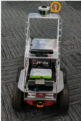
Fig. 8 Our hardware platform, in which the (1) Velodyne VLP-16 3D LiDAR is mounted at 0.8m from the floor, on the top of the Pi-oneer 3-AT robot.
