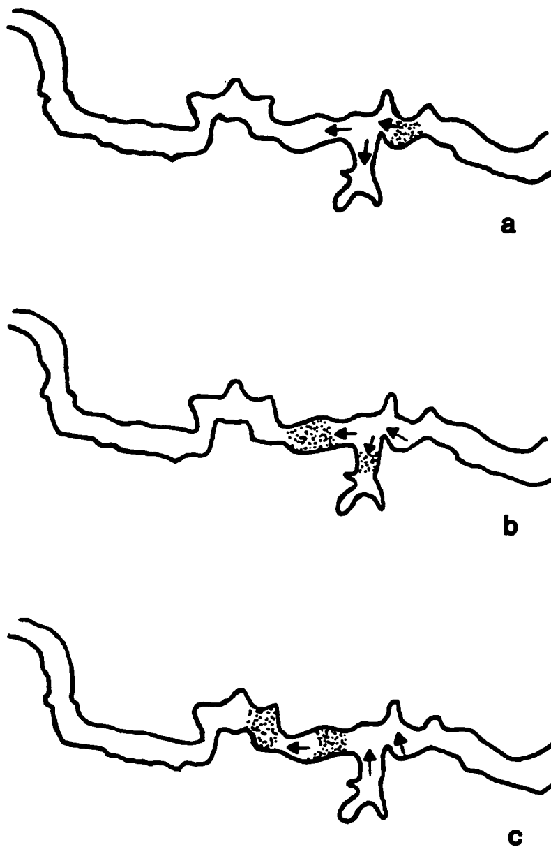
Figure 12. Coastal Plain Estuary with Side Embayments. Dots Represent a Dye Tracer Moving with the Flood Tide (Direction of Arrows) (after Fischer et al., 1979).
