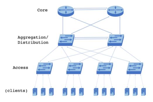
Cisco's Nexus Layer 3 switches are dense enough to allow for design flexibility, especially in data centers, and thus the Core and Aggregation/Distribution layers can be combined. This is also known as a Spine and Leaf design:
