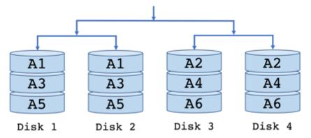
In a RAID 0+1, storage blocks are also mirrored or saved twice in disk drives groups in alternating pairs of drives:
