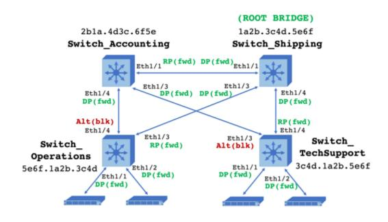
Switch\_Shipping is the root bridge and its Ethernet 1/1, Ethernet 1/3, and Ethernet 1/4 interfaces are designated ports in RSTP and will be forwarding frames.
