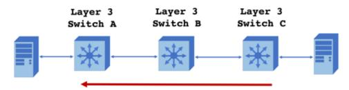
1. Switch C now knows that to reach switch A it has to first send packets to switch B, and so Switch C tells Switch B about a route from Switch C to reach Switch A. So Switch B now thinks it has two routes to get to A: 1) from B to A, and 2) from C to A
