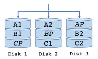
In a RAID 6 configuration, the storage block parity is stored on two drives, the array can now lose two drives and still have the storage block rebuilt based on the parity information:
