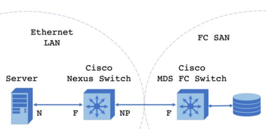
When the Cisco Nexus switch is running in NPV mode, it does not require an FCID and forwards all FC frames to the Cisco MDS switch which is running in NPIV mode.
