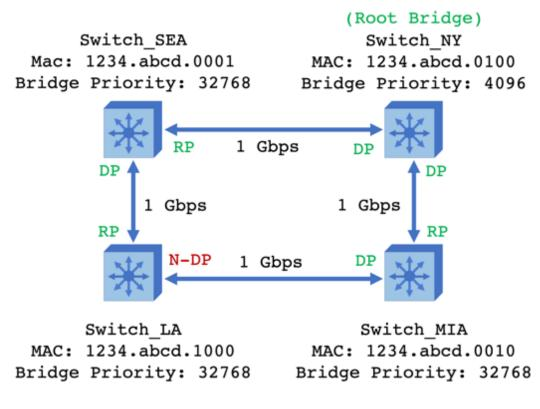
DP = Designated Port (forwards data frames and BPDUs) RP = Root Port (forwards data frames and BPDUs) N-DP = Non-Designated Port (blocks and <u>does not forward frames</u> but will forward BPDUs) 23. These switches have Spanning Tree Protocol enabled, which one will be elected the root bridge?
