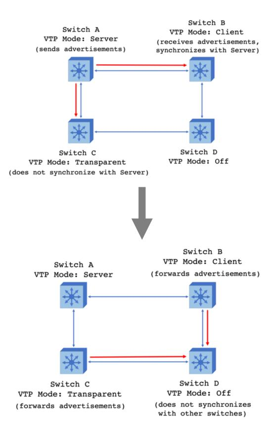
And so, matching the VTP modes to the switch's functions and abilities in that mode:
