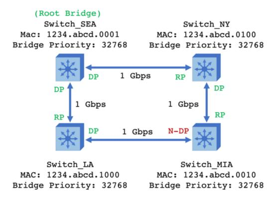
DP = Designated Port (forwards data frames and BPDUs) RP = Root Port (forwards data frames and BPDUs) N-DP = Non-Designated Port (blocks and <u>does not forward frames</u> but will forward BPDUs) Note, when there is a STP cost tie, like when the links from non-root bridges are the same speed and there are an equal number of links between the non-root bridge and the root bridge, then the tie breaker is the lowest BID of the connected switches.
