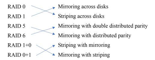
These are the most common Redundant Array of Independent Disks (RAID) configurations (RAID 2, 3, and 4 are not used often), with RAID 6 probably being the most cost effective in larger arrays. Parity is an error correction method where information on a failed hard drive can be rebuilt on a replacement drive.
