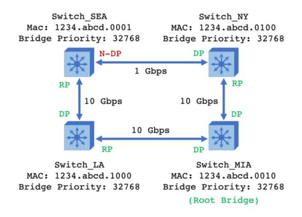
24. In this example, refer to the diagram below and use the Command Line Interface (CLI) on each switch to determine which switch is the Rapid Spanning Tree Protocol root bridge on VLAN 1:
