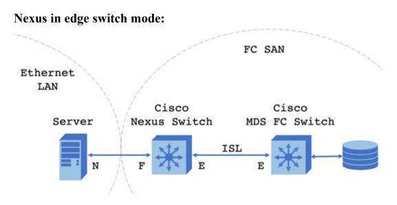
The Cisco Nexus switch is actively processing FC frames (as well as Ethernet frames), and so requires an FCID, an FC domain only has 239 FCIDs.
