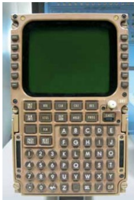
Figure3. Boeing's Control Display Unit (CDU) from "Contribution of Flight Systems to Performance-Based Navigation" (Miller, 2009)
