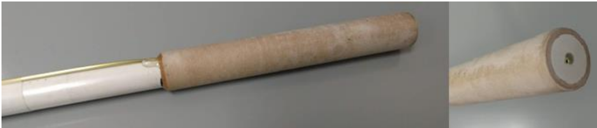
Figure 13: Second dummy sting with cavity pressure tap.
