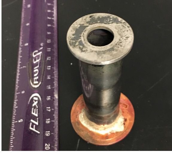
FIG. 18: A photograph of a gasket that was specially created to block scattered light.
