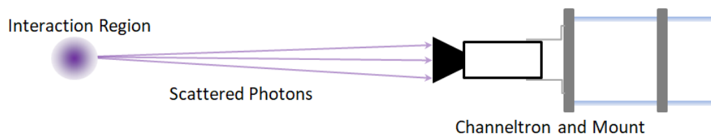
FIG. 29: A diagram showing resonant UV photons scattering out of the interaction region and into the Channeltron.
