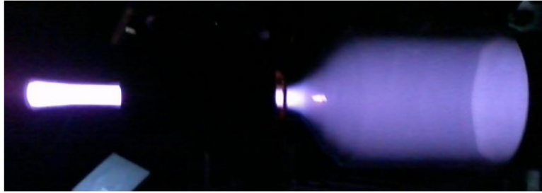
FIG. 24: A photograph taken at the FEL, during the ionization test. It shows the glass tube that was mounted to the front of the beam machine. You can clearly see the glow from the RF discharge. The dark section in the middle is the shielding around the RF coils. In this photo, krypton gas is propagating from left to right. Metastable krypton atoms excited in the RF plasma continue into the chamber and the detection region, not shown in the picture.
