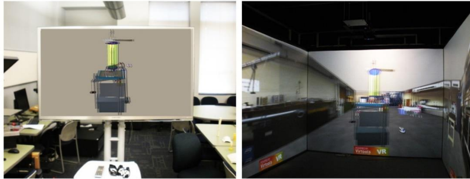
Fig. 15. Virtual Jet-force Experiment on the 3D TV (Left) and the CAVE (Right) System.
