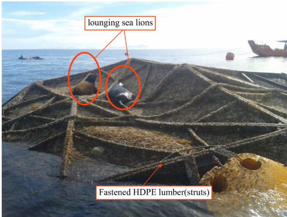
Figure 4.1. Buckled Aquapod cage made from HDPE lumber and netting (covered with biofouling) with two lounging sea lions on the exposed struts (InnovaSea Systems 2015).
