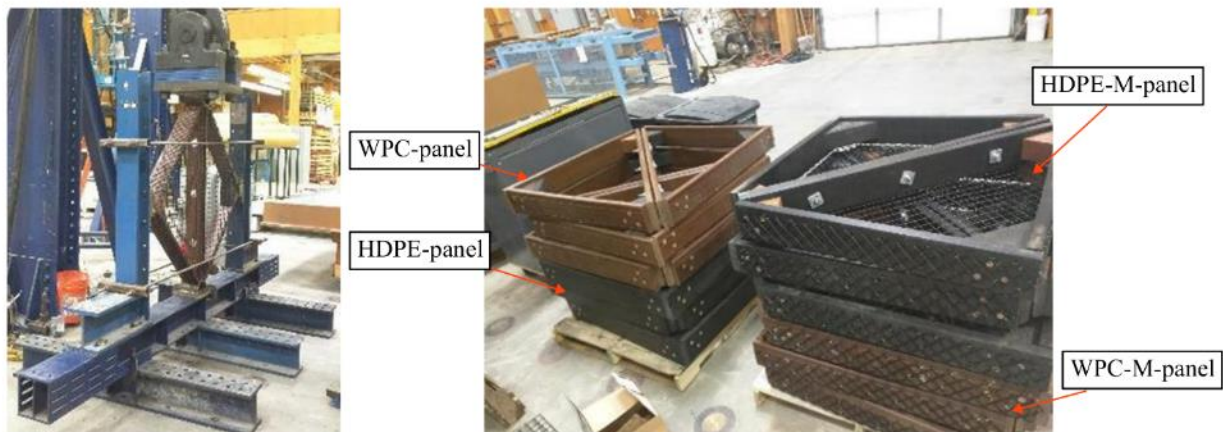
Figure 5.3. (Left) the test frame and the buckling test setup, (right) the WPC and HDPE connected triangular panels with and without metallic mesh.
