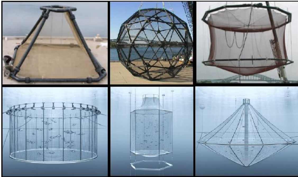
Figure 1.2. Types of aquaculture cages. Clockwise from top left: prototype gravity system, AquaPod net pen, Ocean Cage Aquaculture Technology (OCAT) cage, gravity-type flexible cage, tension-leg system, and rigid-frame fish cage (Vandenbroucke & Metzlauff 2013).
