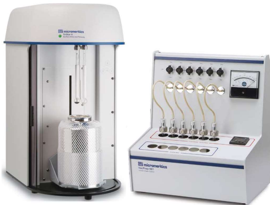
Figure 4.2 Micromeritics TRISTAR II 3020 used for determination of specific surface areas.
