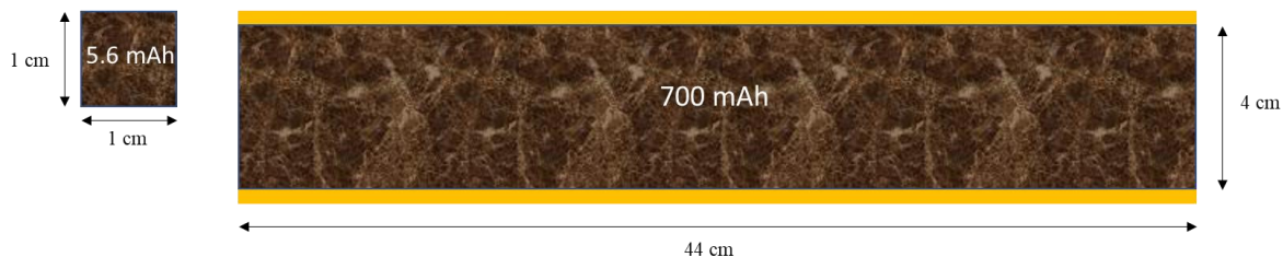
Figure 5.17. Schematic of anode electrode
