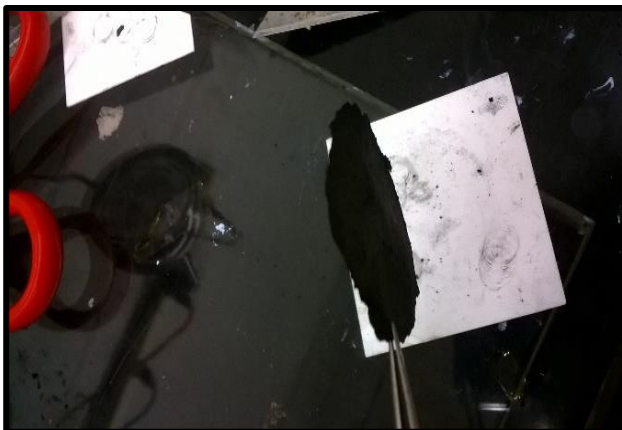
Figure 3.8. Free standing electrode made of activated carbon
