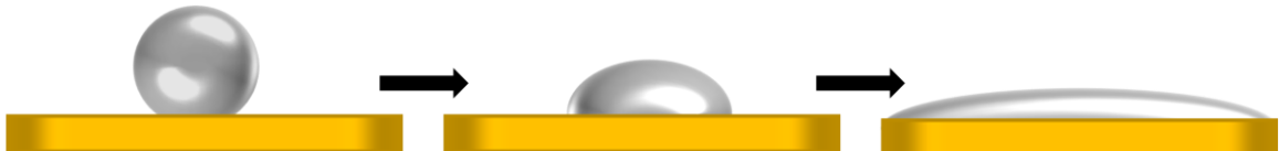
Figure 5.7 Ga film formation during LPE experiments. A Ga film with varying thickness is formed on top of the substrate due to the incorporation of nitrogen into the melt.
