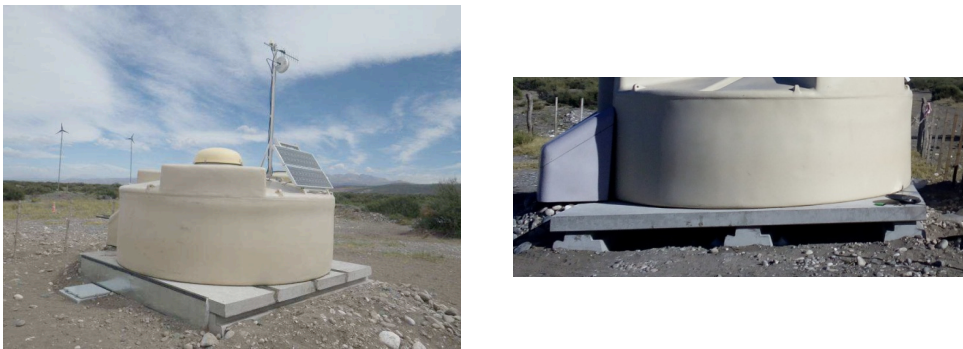
Figure 5: (left) Pierre Auger Observatory water-Cherenkov Detector ( Tierra del Fuego ) with two RPCs below, inside the concrete precast. (right) Detail of the concrete precast while it is open on the side.
