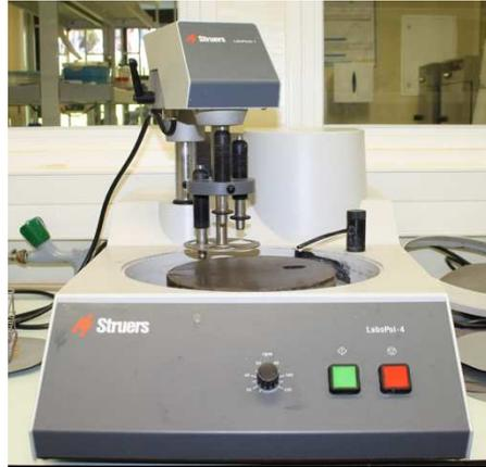
Figura 12 - Máquina Polidora (LaboPol-4, Struers, A/S, Ballerup, Denmark)
