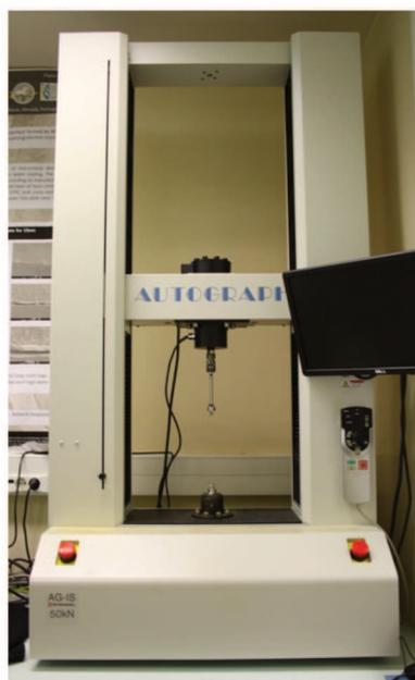
Figura 19 - Máquina de testes universal (Shimadzu Autograph AG-IS, Tokyo, Japan)
