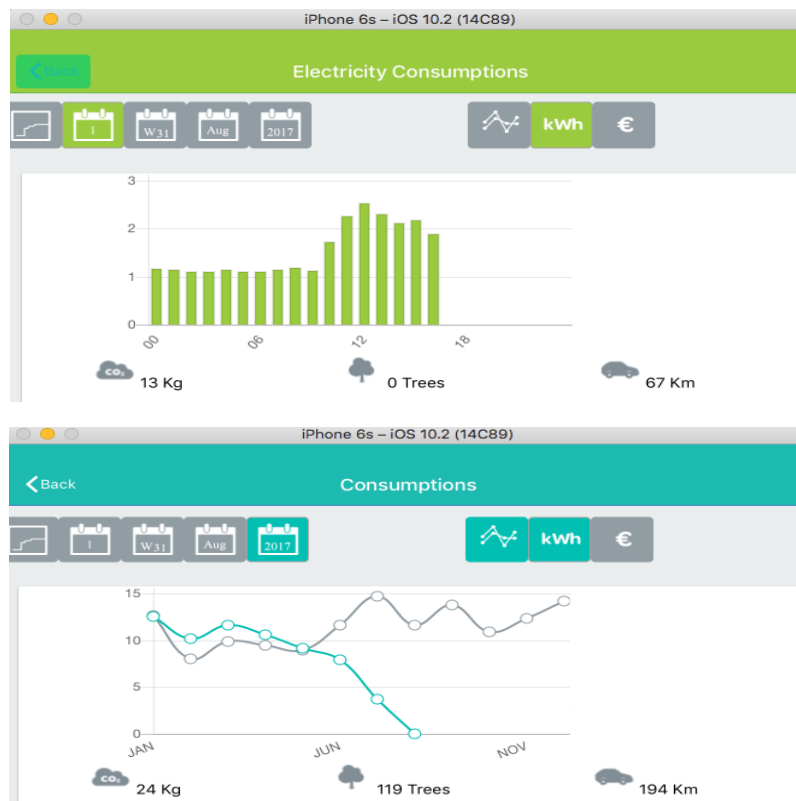
Figure 5-31 Snapshot from iOS where Consumption module for electricity and plugs is presented respectively.
