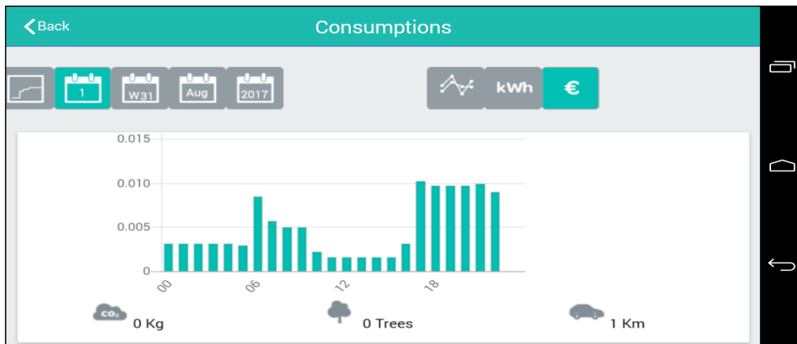
Figure 5-17 Consumption module of one of the plugs where chart.js has been implemented
