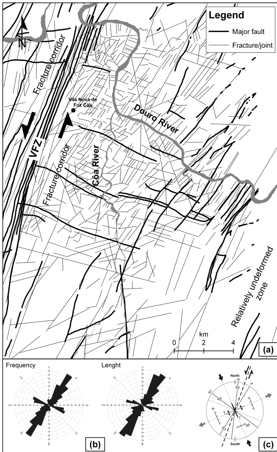
Fig. 3. Lineation map of the study area. The lineations detected by visual interpretation of all the processed Landsat images were reported. Thick lines represent the major faults where the arrows indicate sense of slip and detected from the literature, supplemented by field surveys. The thin lines are fractures and joints detected by satellite images and, in some cases, are supplemented by field surveys. VFZ = Vilarica Fault Zone (a); rose diagrams with class interval of 10 degrees and population of 705 showing the statistical distribution based on lineament length and frequency detected by the satellite images analysis (b); arrangement of structures associated with a NNE-SSW sinistral shear zone (the VFZ) for the study region. R = synthetic riedel shears; R1 = antithetic riedel shears; N = normal faults; F = fold axis; RF = reverse faults; P = secondary synthetic shears; T = tensional fractures; short black arrows = sigma 1 (maximum compressive stress); short grey arrows = sigma 3 (maximum tensile stress) (c).
