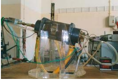
Fig. 10. FFC NMR air cored magnet (solenoid type).
