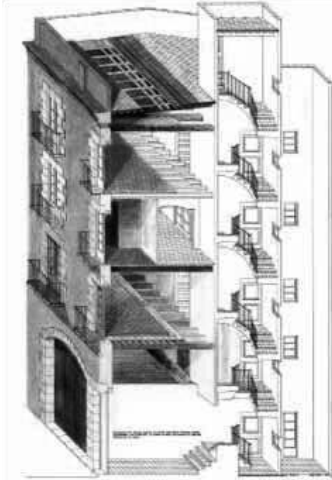
Figure 3. Interpretation of a project conducted by Josep Renau and Francesc Mestres (master builders) in 1787. (Rosell Colomina, 1996: 300) that reflects well the new type of building
