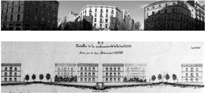
Figure 7. The so called "Cerdà houses" (named after the owner, not the planner) were among the first to be built in the new city. But, as you can see in the picture below, the building volume is superior to that proposed by Cerdà himself (Cerdà, 1859)
