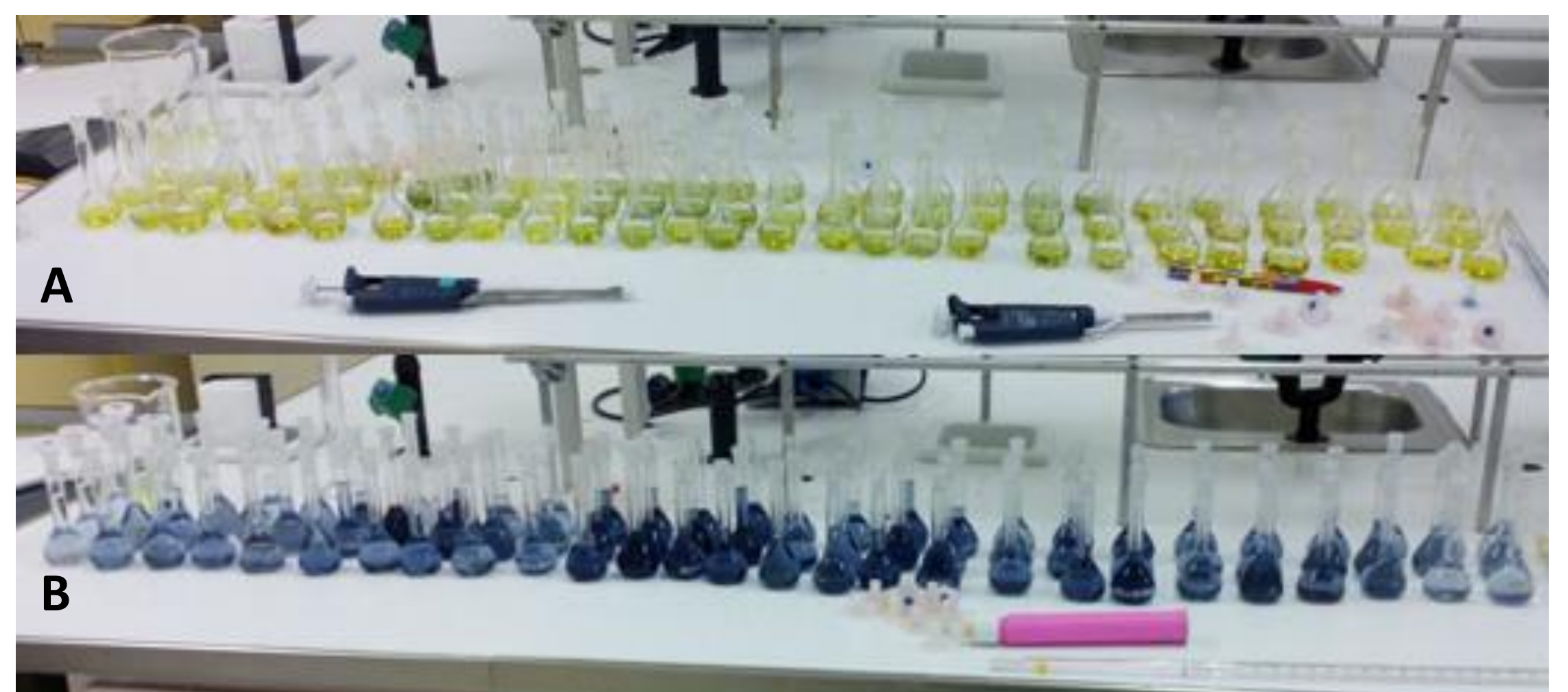
Fig. 2 – Samples before (A) and after (B) the Folin-Ciocalteu reaction
