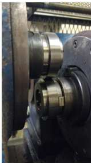
Figure 3 (a) Image of test discs mounted on the SUROS tester.
