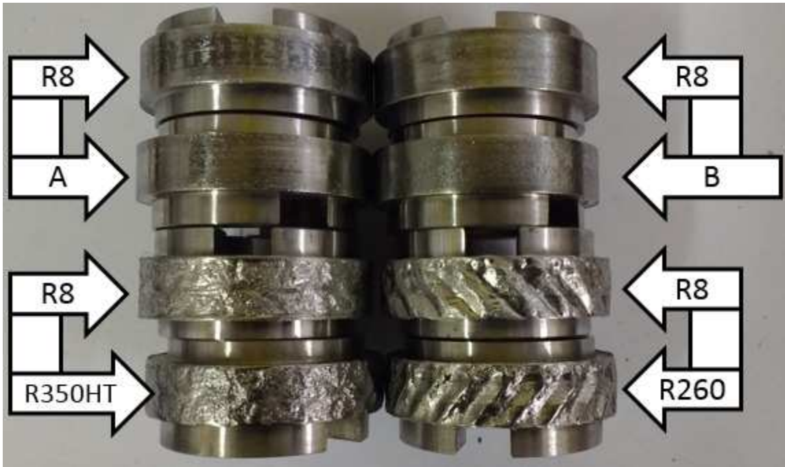
Figure 13 Image of wheel and rail discs after testing at 20% slip.
