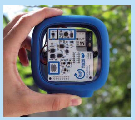
a Wi-Fi connection, or it can store the data on a MicroSD card. The SCK has a low power consumption, making it ideal for placement on balconies and windowsills. The device can be charged either by solar panel or mini-USB connector.
