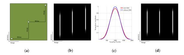
**Figure 5.** Demonstration of the influence of DRR: (**a**) shows a scene with three target points located at different range and azimuth positions; (**b**) illustrates the symmetrical shift of the azimuth signal after pre-processing with DRR error; (**c**) shows the scaling effect of the azimuth signal after pre-processing with DRR error; (**d**) the result of pre-processing without DRR error.
