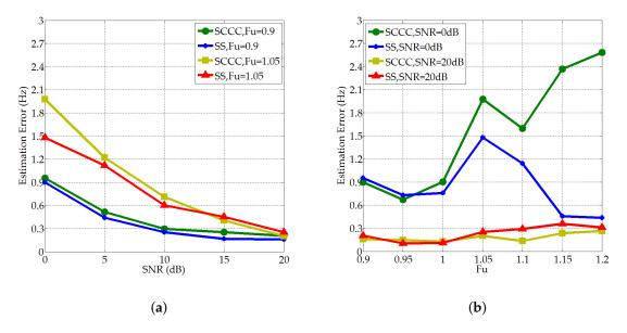
Figure 13. The performance of CDC error estimation method versus SNR (a) and Fu (b).
