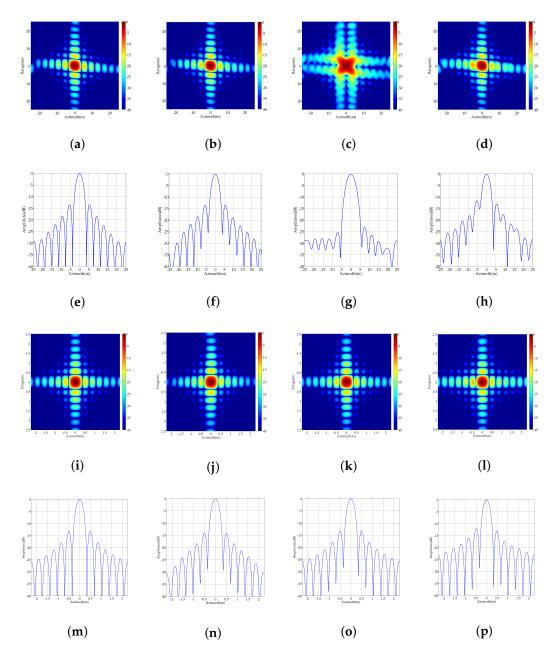
**Figure 11.** Imaging results of multi-channel TOPSAR without errors (**a**), with DRR error (**b**), CDC error (**c**), phase inconsistency errors (**d**–**h**) are corresponding azimuth profiles. Imaging results of multi-channel sliding spotlight SAR without errors (**i**), with DRR error (**j**), CDC error (**k**), phase inconsistency errors (**l**–**p**) are corresponding azimuth profiles.
