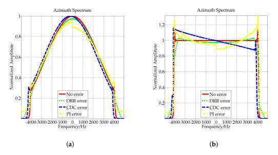
**Figure 10.** Azimuth signals of multi-channel TOPSAR after pre-processing: (**a**) shows the amplitude of signals with DRR error (dotted green line), CDC error (dashed blue line), phase inconsistency errors (dash-dot yellow line) and without error (red line); (**b**) shows the amplitude of the signals after antenna correction.
