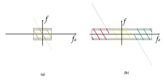
**Figure 7.** The Doppler frequency aliasing in multi-channel strip-map SAR (**a**) and multi-channel BS-SAR (**b**). The three colors represent three targets in azimuth. f and  $f_a$  denote the baseband frequency and physical frequency, respectively.
