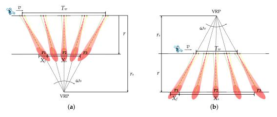
**Figure 2.** Multi-channel sliding spotlight SAR and multi-channel TOPSAR. (**a**) is the multi-channel sliding spotlight and (**b**) is the multi-channel TOPSAR. Three different colors (green, red and yellow) in the figure represent three different channels.
