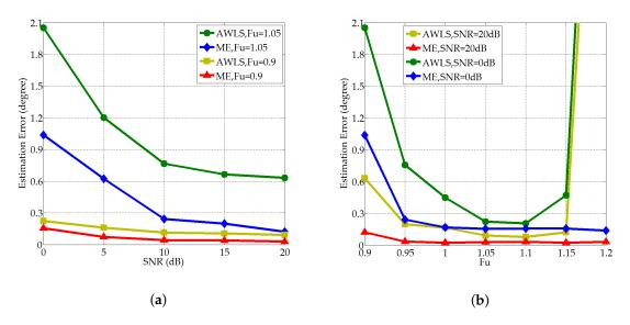
Figure 14. The performance of CDC error estimation method versus SNR (a) and Fu (b).
