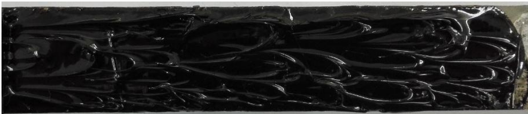
10 11 Figure 7. Failure surface of specimens prepared with G2 aggregates in dry condition 12
