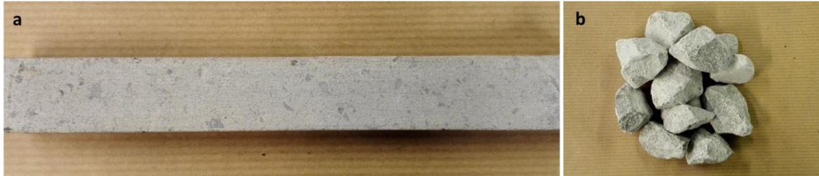
Figure 1. Aggregate substrate and coarse aggregates: (a) substrate must be prepared from large boulders, while (b) coarse aggregates are readily available in most labs.
