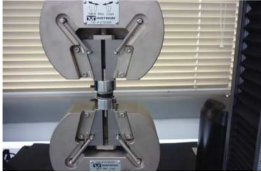
Figure 2. Adhesion strength test set-up.
