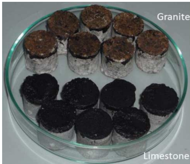
Figure 7. Sample loci of failure for moisture-induced damage in aggregate–asphalt mastic systems showing effect of conditioning time and aggregate type. All specimens were conditioned in water for up to 7 days in water at 20°C before tensile testing. Top: granite specimen showing complete stripping (adhesive failure) of mastic from aggregate. Lower: no significant stripping observed in limestone aggregate bonds (mainly cohesive failure).
