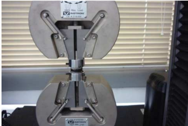
Figure 2. Adhesion strength test set-up.
