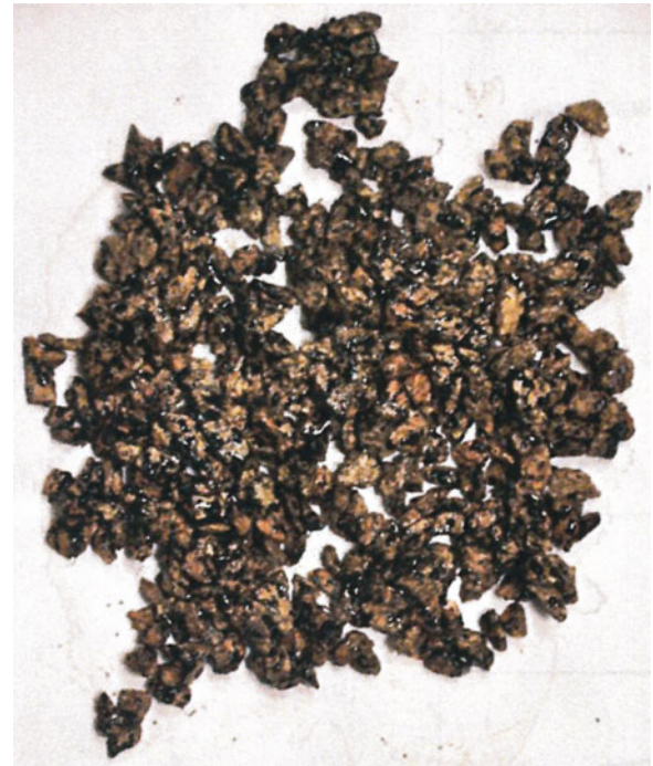
Figure 5. BWT results showing G3 granite mixture almost stripped of the 40/60 pen binder used.
