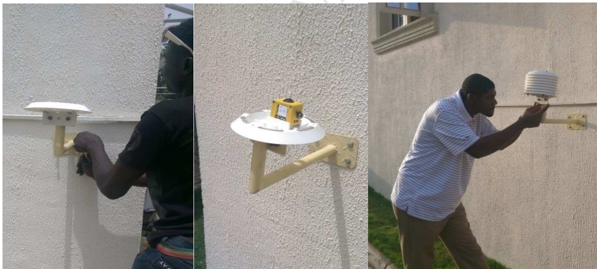
Figure 4: Installation with radiation shield of Tinytag data logger used to measure outdoor environmental variables
