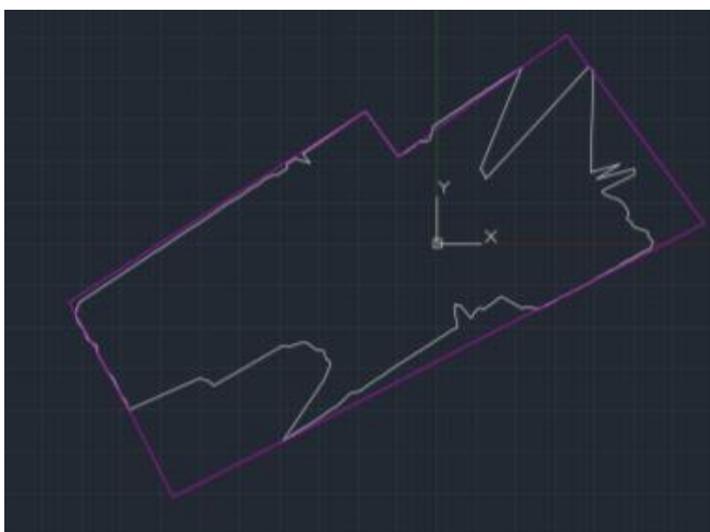
Figure 54 – Edited 2D AutoCAD model dining room and kitchen of flat using point cloud data from excel using collected by RPLidar 360 Robot Laser Scanner
