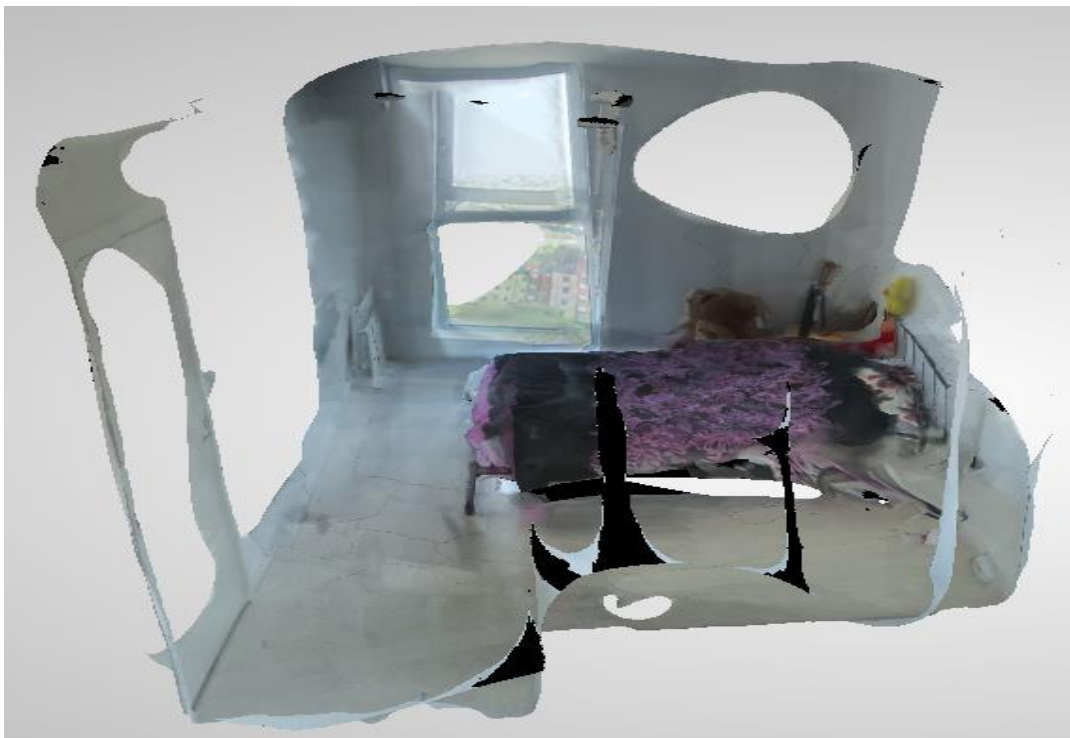
Figure 35– side view 3D models from photographs of flat using Recap 360
