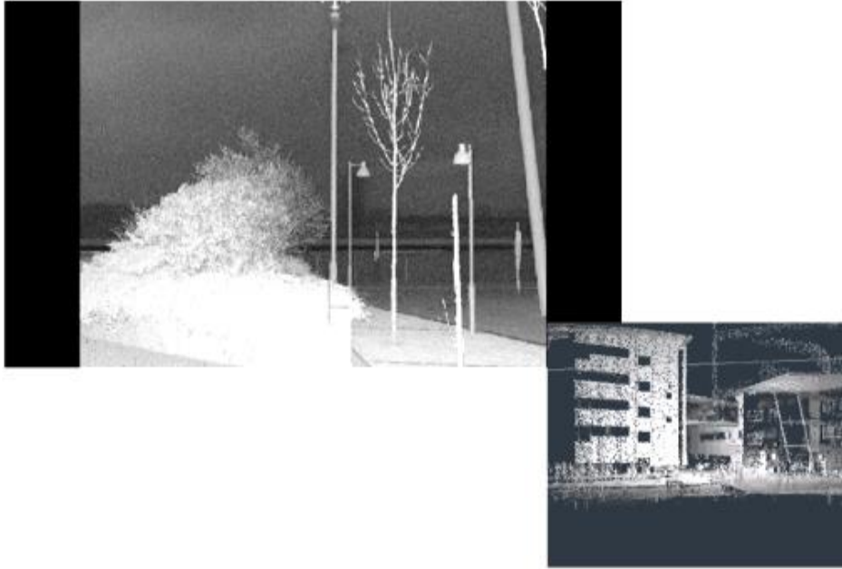
Figure 7 – view of Point Cloud of Knowledge Dock at University of East London from within model created using Recap software from data collected by a Faro laser scanner.
