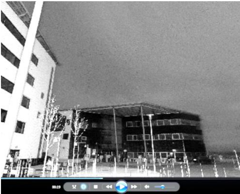
Figure 7 – view of Point Cloud of Knowledge Dock at University of East London from within model created using Recap software from data collected by a Faro laser scanner.
