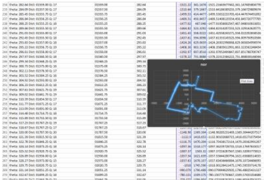
Figure 46– Point Cloud data dining room and kitchen of flat in excel using ultra grabber software collected by RP Lidar 360 Robot Laser Scanner
