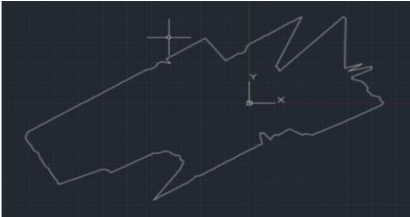
Figure 53 – 2D AutoCAD model corridor of flat using point cloud data from excel using collected by RP Lidar 360 Robot Laser Scanner
