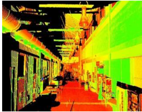
Figure 5: East Building Atrium at University of East London using Leica Scanner and Cyclone Software (also from Leica)
