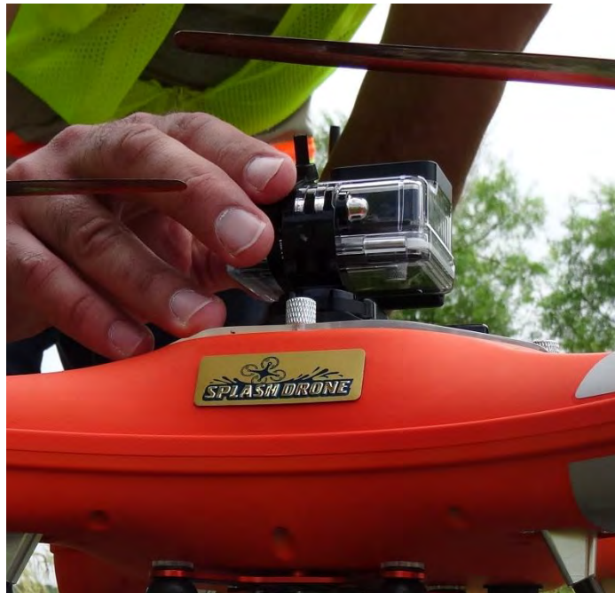
Figure 52: GoPro camera mounted onboard the Mariner 2 Splash UAV, about to collect imagery of the underside of the northbound US-31/ White River bridge.
