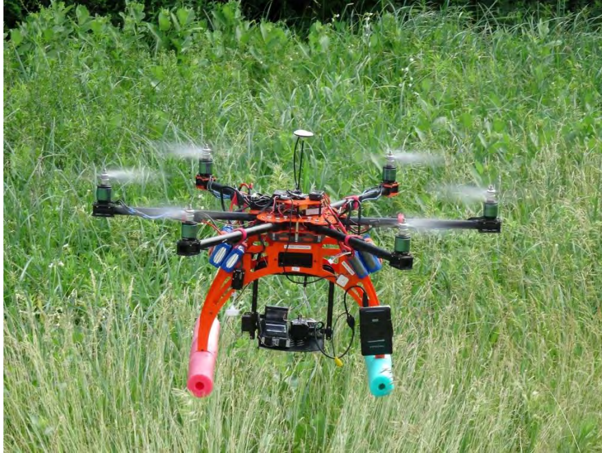
Figure 25: A Bergen Hexacopter shortly after take-off, about to collect thermal imagery of the US-31 road corridor with dual FLIR cameras.
