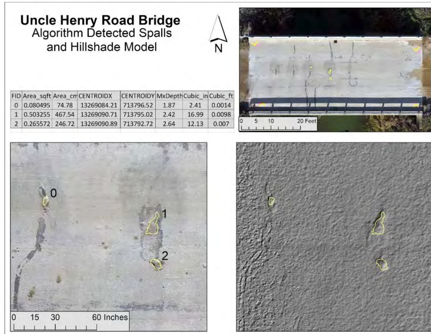
Figure 81: Uncle Henry detected spalls and associated attribute data shown with orthophoto and hillshade layers.
