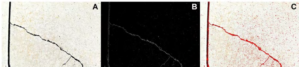
Figure 98: A. The original image of concrete containing cracks. B. Output from Matlab code where white is “detected” crack. C. Final merged product over original image.
