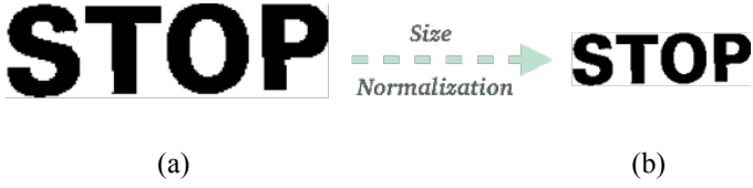
Fig. 4. Size normalization of binarized images. (a) Original image with 232×831 pixels. (b) Normalized image with 50×170 pixels.
