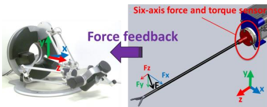
Figure 5. Force sensing and its realization in Omega 7.
