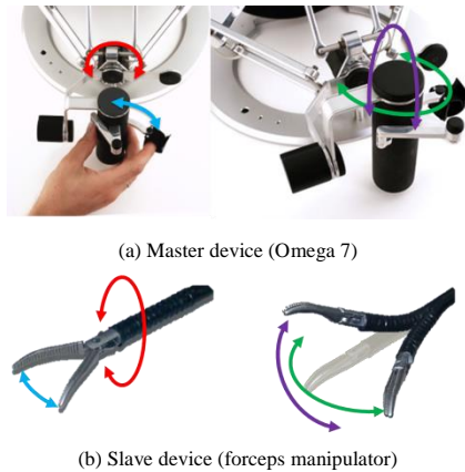
Fig. 4. Manipulations of Omega 7 and forceps manipulator.
