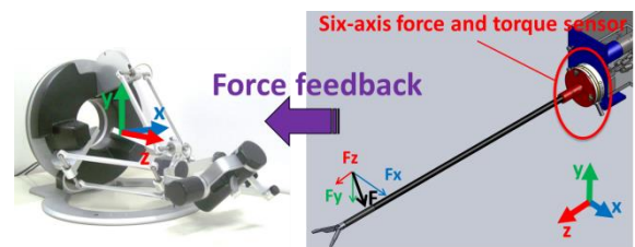
Fig. 5. Force sensing and its realization in Omega 7.
