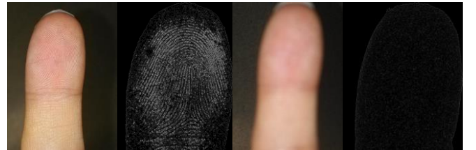
Fig. 12. Clear image with its Sobel edge, blur image with its Sobel edge
