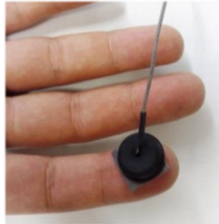
(a) Attachment place for the bidirectional microphone used as vibration sensor
