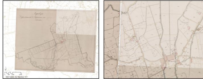
Fig. 6. A Napoleonic Cadastral map (1811) geo-referenced against the modern topographic maps. On the right: the zoom shows the Napoleonic map plotted against the modern topographic map.
