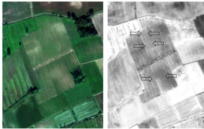
Fig. 4. The use of MSAVI2 (right) allows for visualising linear traces that are not visible in the True colour (left) MIVIS data.
