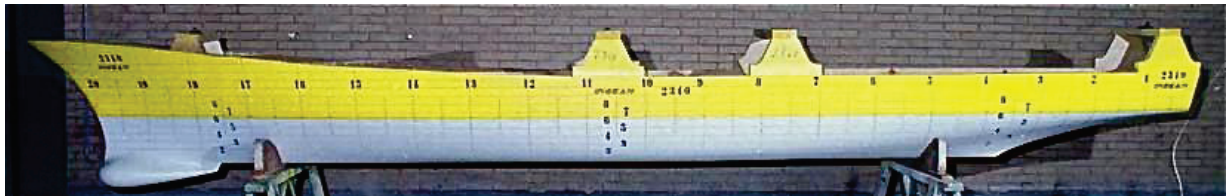
Fig. 2: A 5.720 m length model of the DTMB 5415 (CNR-INSEAN model 2340)
